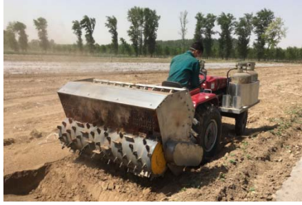
Appendix A The second generation SFD machine disinfesting soil.
