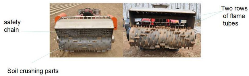
Appendix B Fine rotary tillage device and high temperature generating equipment on the second generation SFD machine.
