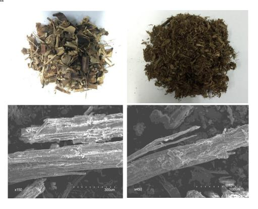
Surface appearance and the scanning electron microscope (SEM) images of wheat and cotton straws before (*left*) or after (*right*) steam explosion (the images of other crop straws are similar thus not shown).
