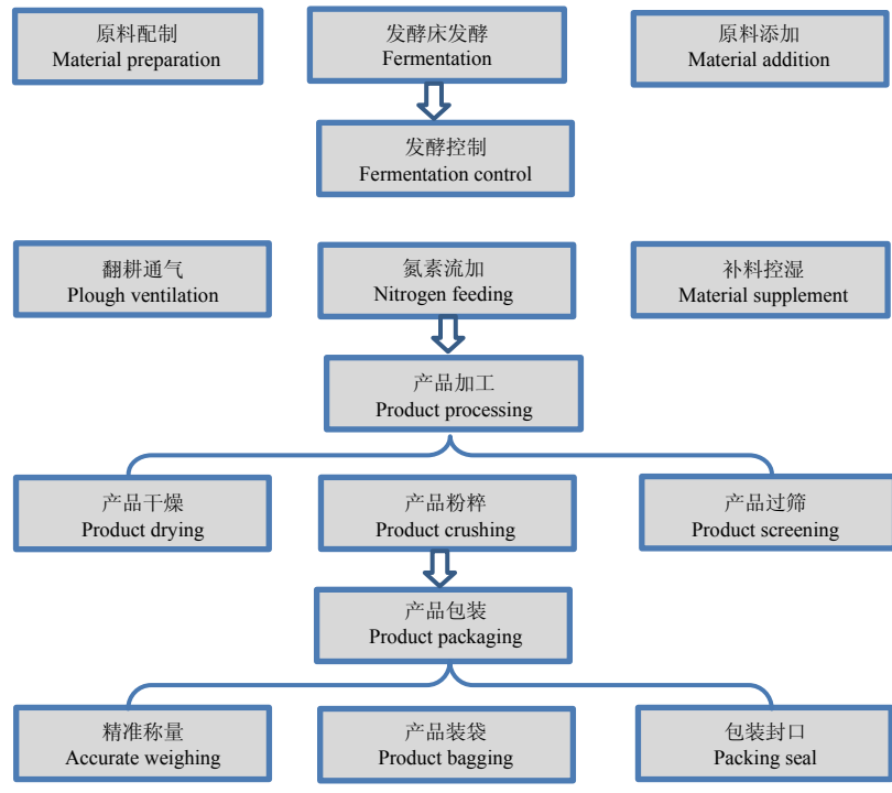
图 1 整合微生物组菌剂的生产工艺 Fig. 1 Production process of the integrated microbiome agent
